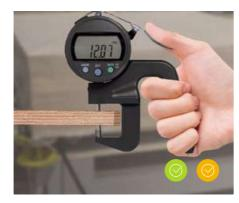
**THICKNESS TOLERANCES ±0.2 MM\***
